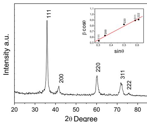
Fig. 2. XRD of sintered SiC ceramic at 1500 °C for 1 min (the inset exemplifies the Williamson-Hall plot).
