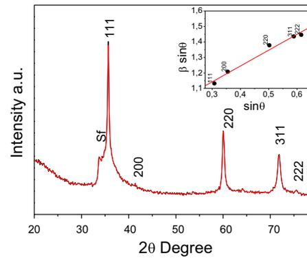
Fig. 1. XRD of as-prepared SiC powder, (SF-stacking fault) (the inset exemplifies the Williamson–Hall plot).
