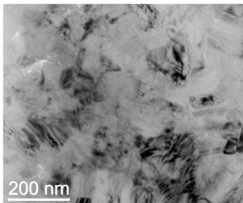
Fig. 3. Transmission electron micrograph of SiC sintered at 1500 °C for 1 min.
