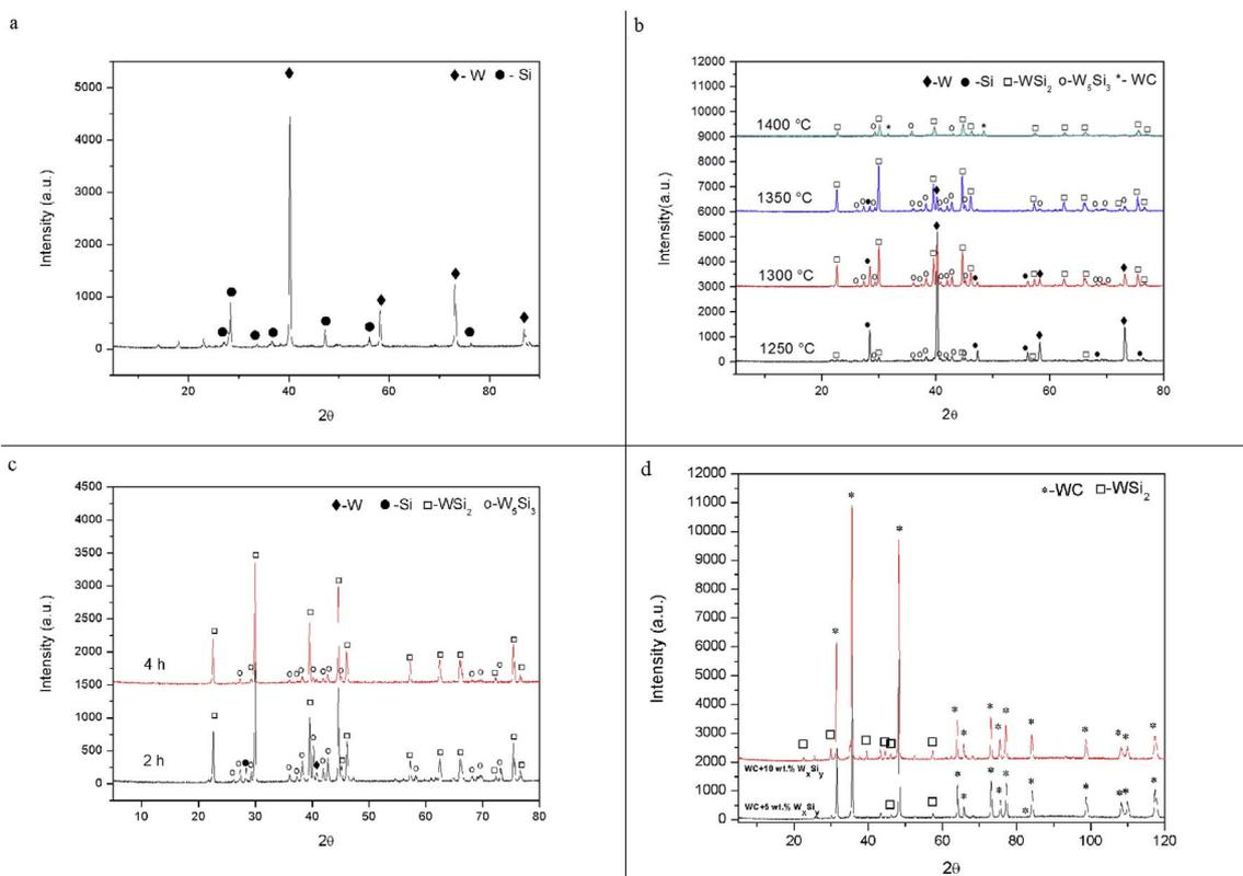
Fig. 1. a) XRD pattern of starting powders after homogenization procedure b) XRD patterns of samples obtained after heating at different temperatures for 2 h in an argon atmosphere. c) XRD patterns of samples obtained at 1350 °C for different amounts of heating time.
