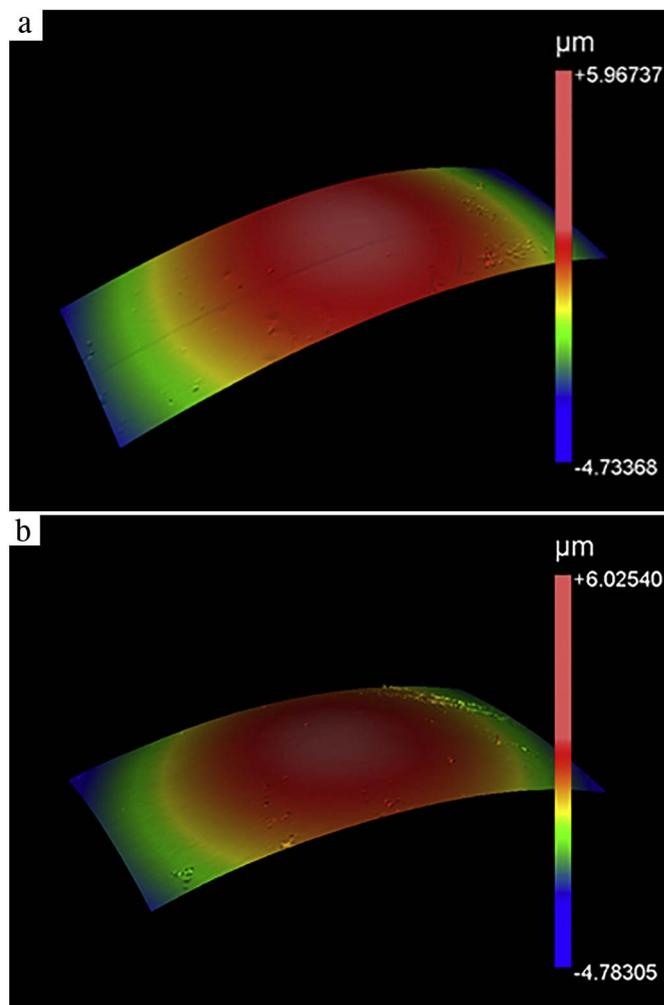
Fig. 4. 3D projection of 5% WSi surface topography after final cavitation.
