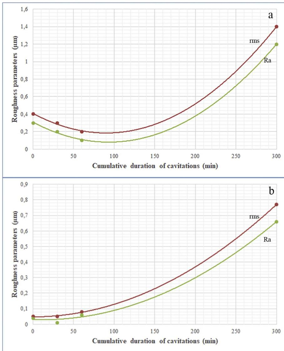
Fig. 5. Change in surface roughness parameters during cavitation erosion testing for sintered samples: a) WC + 5 wt% W<sub>x</sub>Si<sub>y</sub>, b) WC + 10 wt% W<sub>x</sub>Si<sub>y</sub>.
