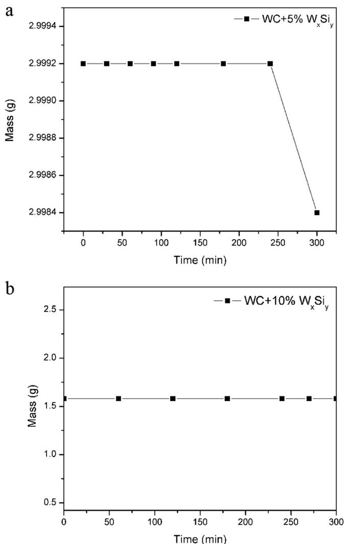
Fig. 3. Mass loss of sintered samples during the cavitation erosion testing: a) WC + 5 wt % W<sub>x</sub>Si<sub>y</sub>, b) WC + 10 wt% W<sub>x</sub>Si<sub>y</sub>.
