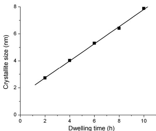
Fig. 2 Crystallite size of SiC of the as-thermolyzed Si–B–C–N ceramic at 1300 °C for various dwelling time (heating rate of 5 °C/min) showing a linear fit.
