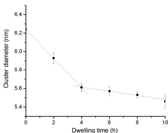
Fig. 5 Cluster size of carbon of the as-thermolyzed Si-B-C-N ceramic at  $1300\text{ }^\circ\text{C}$  for various dwelling time (heating rate of  $5\text{ }^\circ\text{C}/\text{min}$ ) showing change in rate of opening up of bonds in free carbon cluster at 4 h.
