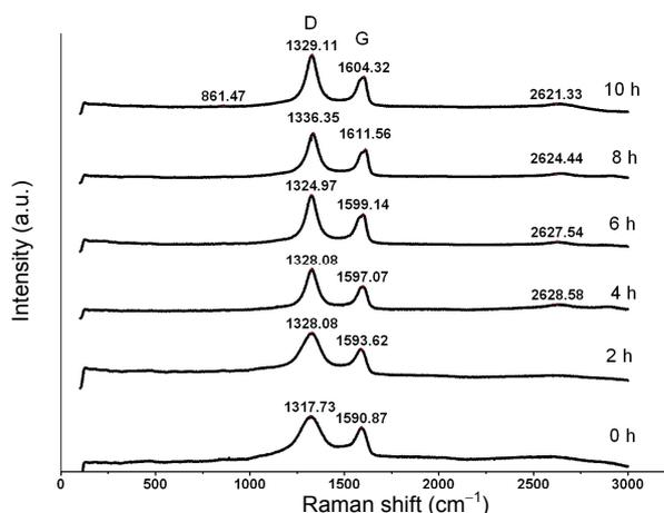
Fig. 4 Raman spectra of the as-thermolyzed Si–B–C–N ceramic at 1300 °C for various dwelling time (heating rate of 5 °C/min).
