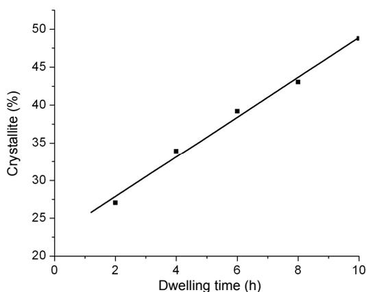
Fig. 3 Percentage of crystallinity in the as-thermolyzed Si–B–C–N ceramic at 1300 °C for various dwelling time (heating rate of 5 °C/min) showing a linear fit.
