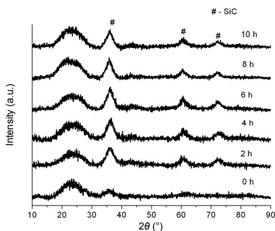
Fig. 1 X-ray diffractograms of the as-thermolyzed Si-B-C-N ceramic at  $1300^\circ\text{C}$  for various dwelling time (heating rate of  $5^\circ\text{C}/\text{min}$ ).
