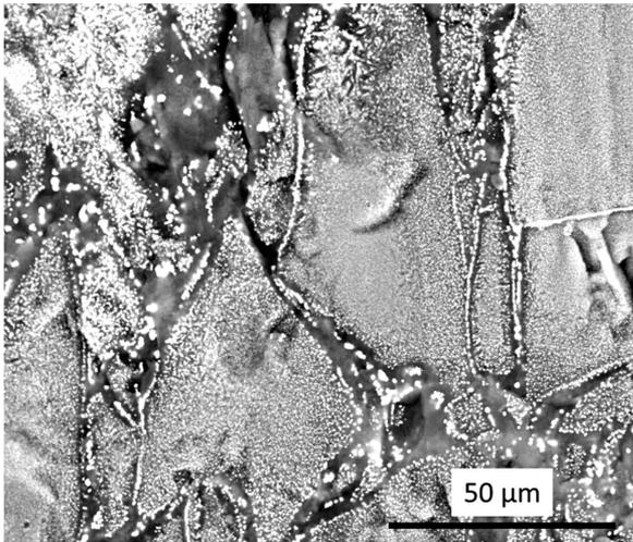
Fig. 1. Back scattered electron micrograph of  $\text{HfO}_2/\text{SiCN}(\text{O})$ . Bright regions indicate enriched regions of  $\text{HfO}_2$ .
