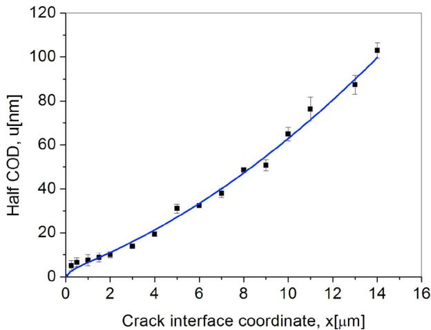
Fig. 4. Half of the crack opening displacement is plotted as a function of crack interface coordinate measured from the crack tip. Solid line shows the fitted line as per Equation 4.
