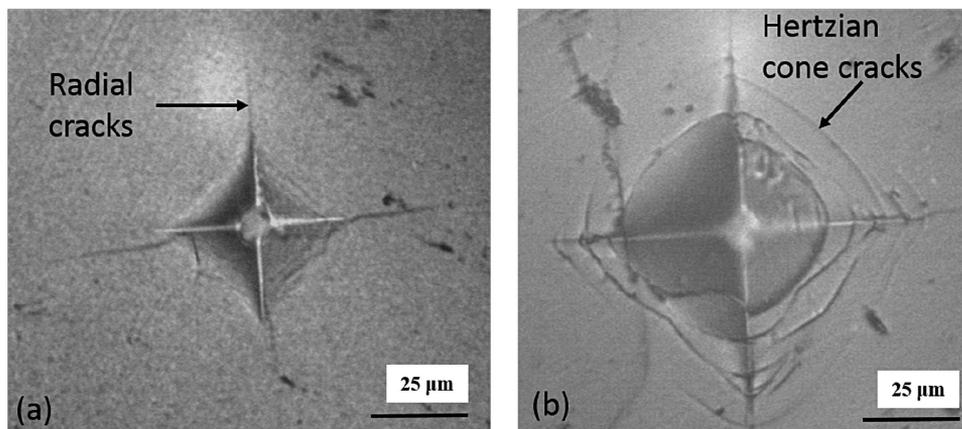
Fig. 2. Crack evolution in (a)  $\text{HfO}_2/\text{SiCN}(\text{O})$  and (b) SiOC PDCs.
