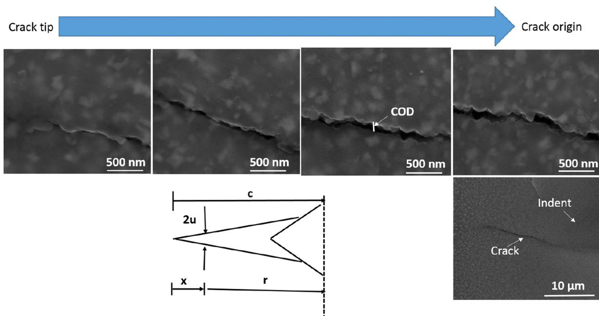
Fig. 3. Crack profile after indentation of HfO<sub>2</sub>/SiCN(O) PDC nanocomposite, showing the COD from the crack tip to the crack origin.
