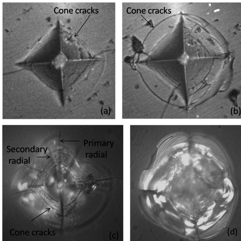
Fig. 6. Optical micrographs indicating the evolution of crack in PECS SiOC (a) at a  $P_{max}$  of 4900 mN; (b) at a  $P_{max}$  of 9800 mN and fused quartz ceramic (c) at a  $P_{max}$  of 4900 mN and (d) at a  $P_{max}$  of 9800 mN.
