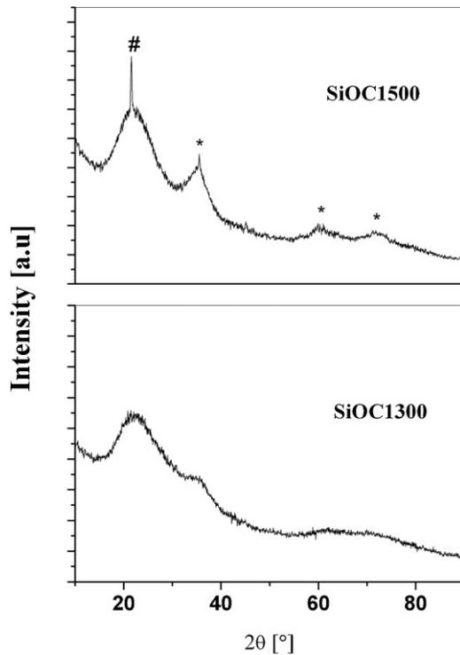
Fig. 1. X-ray diffractograms of the PECS SiOC ceramics: \*, SiC; #, SiO<sub>2</sub>.
