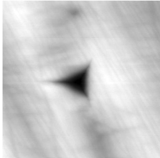
Fig. 4. Scanning probe micrograph of the indent on SiOC1500 at a  $P_{max}$  of 10 mN (image size:  $4 \mu m \times 4 \mu m$ ).
