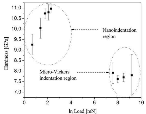
Fig. 5. Variation in hardness with  $\ln$  (load) for SiOC1500.
