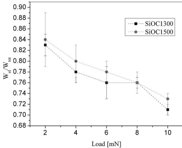
Fig. 3. The evolution of elastic work ratio with indentation load.
