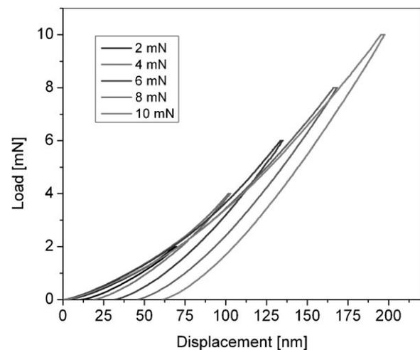
Fig. 2. Load–displacement curves for SiOC1500 subjected to indentation at varied loads between 2 and 10 mN.
